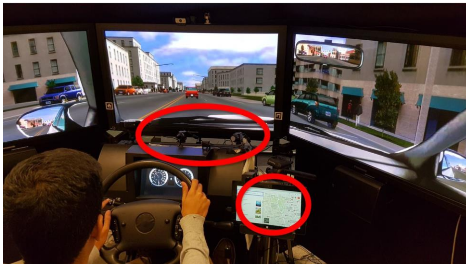
Figure 1: Simulator setup with eye tracker and secondary display highlighted
