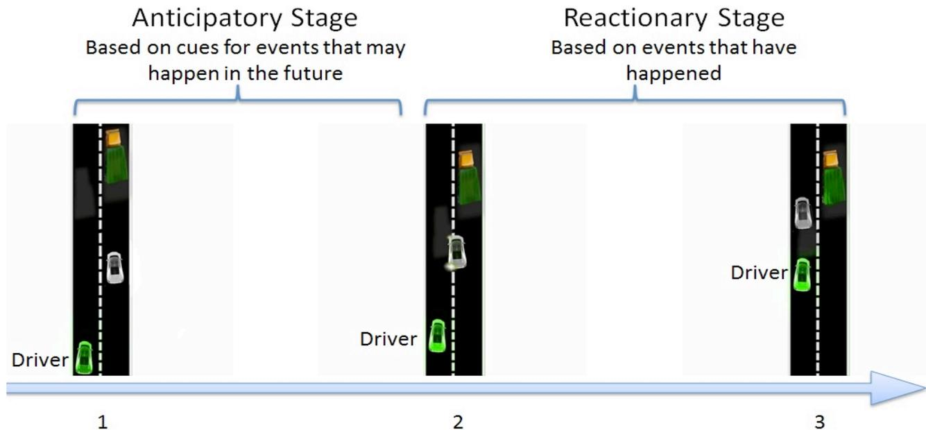
**Figure 1: Anticipatory Scenario - A potential headway conflict for the driver, caused by the lane change of a second car that attempts to overtake a vehicle in its own lane**
