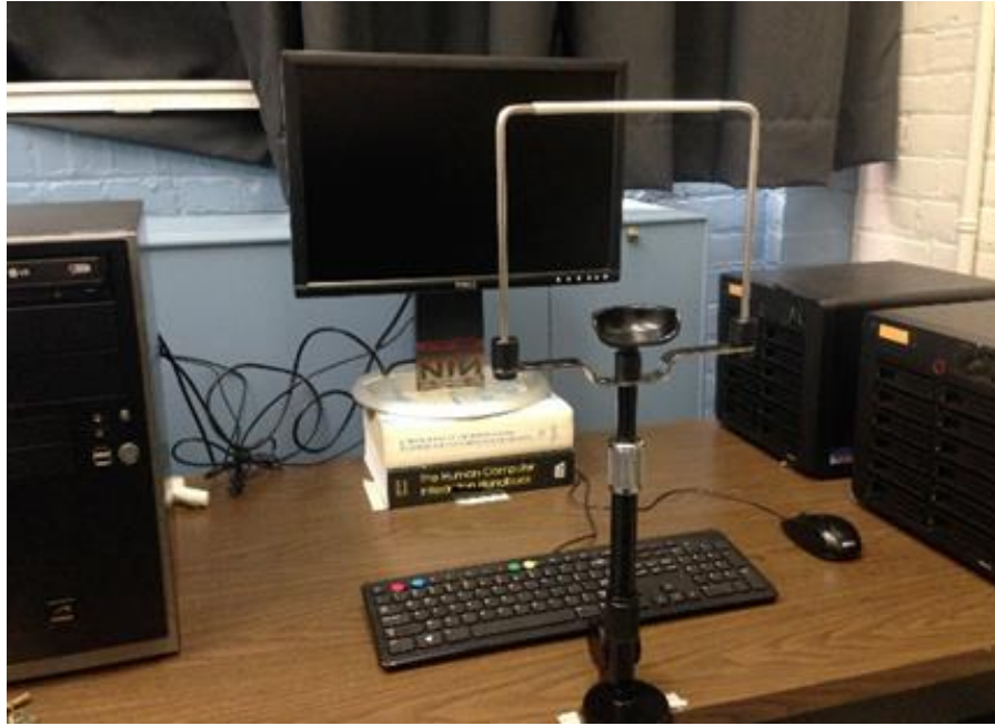
Figure 26: Experimental setup for cognitive tasks. The head/chin rest was used for the flanker task
