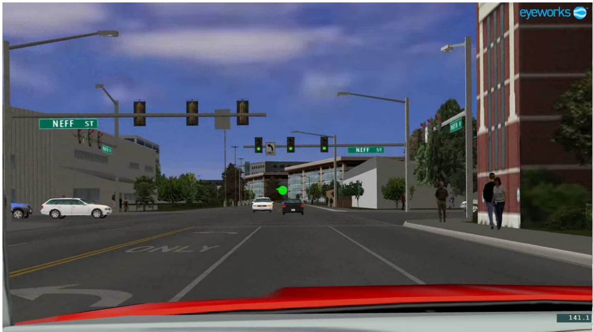
Figure 3: Centre screen simulator display on approach to the intersection with the left-turn vehicle hazard in Drive A for one participant. The green dot and green line represent the participant's gaze location and gaze trail, respectively.
