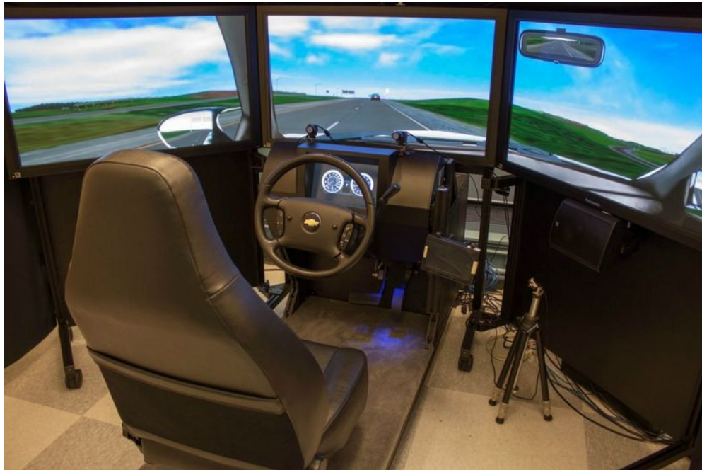
Figure 2: Photograph of the NADS MiniSim simulator used in the experiment. The faceLAB cameras are mounted on the dashboard on either side of the instrument panel.
