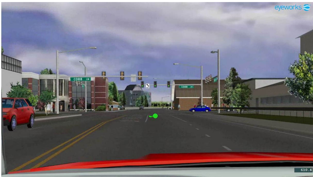
Figure 7: Screen capture of the centre display of the simulator on approach to the right incursion hazard in Drive A for one participant. The green dot and green line represent the participant's gaze location and gaze trail, respectively.
