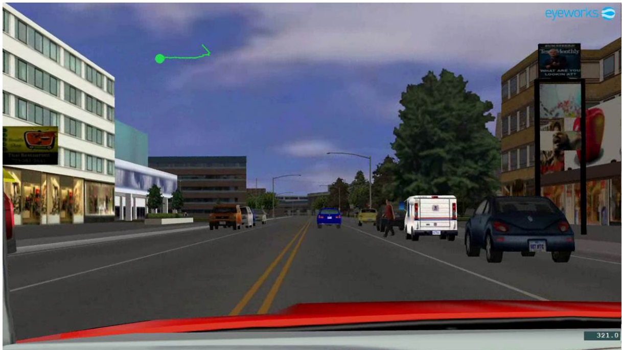
Figure 5: Simulator centre screen display shortly after the presentation of the pedestrian hazard in Drive A for one participant. The green dot and green line represent the participant's gaze location and gaze trail, respectively.
