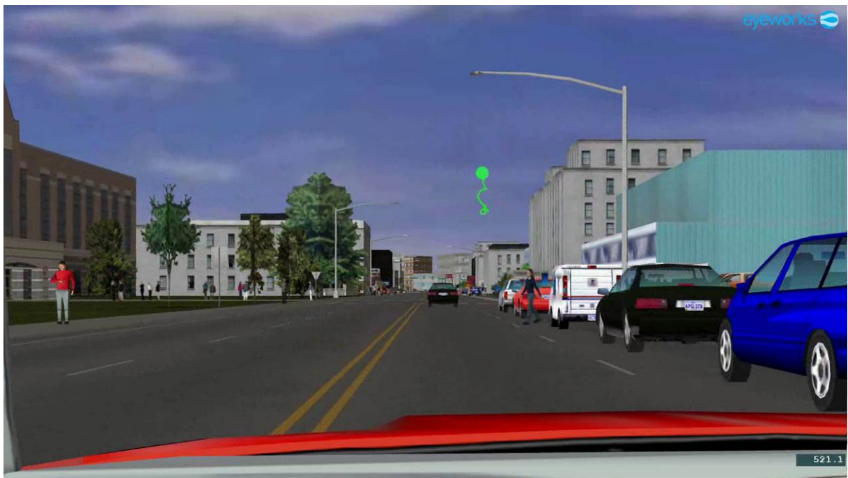
Figure 6: Simulator centre screen display shortly after the presentation of the pedestrian hazard in Drive B for one participant. The green dot and green line represent the participant's gaze location and gaze trail, respectively.
