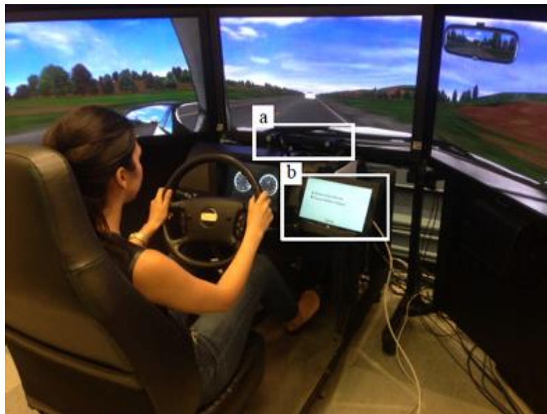
183 Figure 1: University of Toronto NADS MiniSim™ driving simulator with (a) eye-tracking 184 cameras and (b) in-vehicle display
