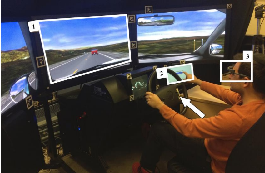
Figure 1. Simulator set up. Arrow indicates the location of the buttons to engage/disengage the automation. (1) Front Screen AOI (2) Non-driving task AOI; task presented on a Surface Pro 2 tablet (3) Dikablis eyetracker
