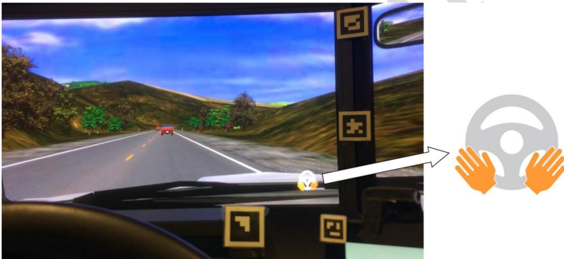
Figure 4. The view of the TOR display on the front screen in the simulator
