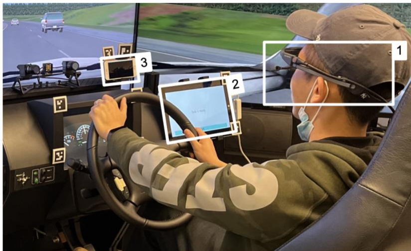
Figure 25. Study 3 experimental setup. 1 = Ergoneers Dikablis eye tracker. 2 = Surface tablet which displayed the training videos (before experimental drives) and secondary task (during experimental drives). 3 = smartphone which displayed the visual component of the attention monitoring system.
