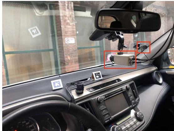
Figure 6 Camera facing the front scene (left) and facing the driver seat (right)
