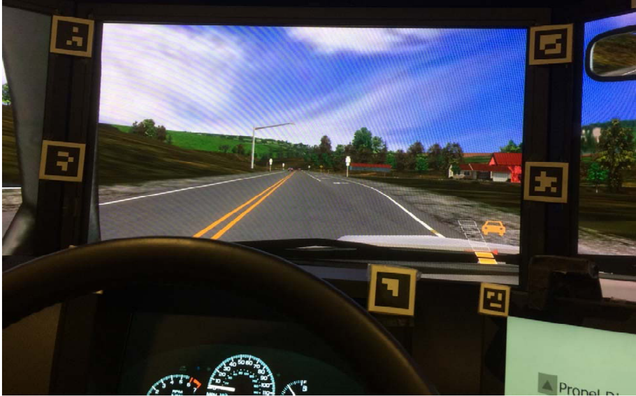
Figure 7: View of the reliability display at Level 2 on the center monitor from the perspective of the driver. The vehicle is at an intersection here. The reliability display is at the bottom right of the screen.
