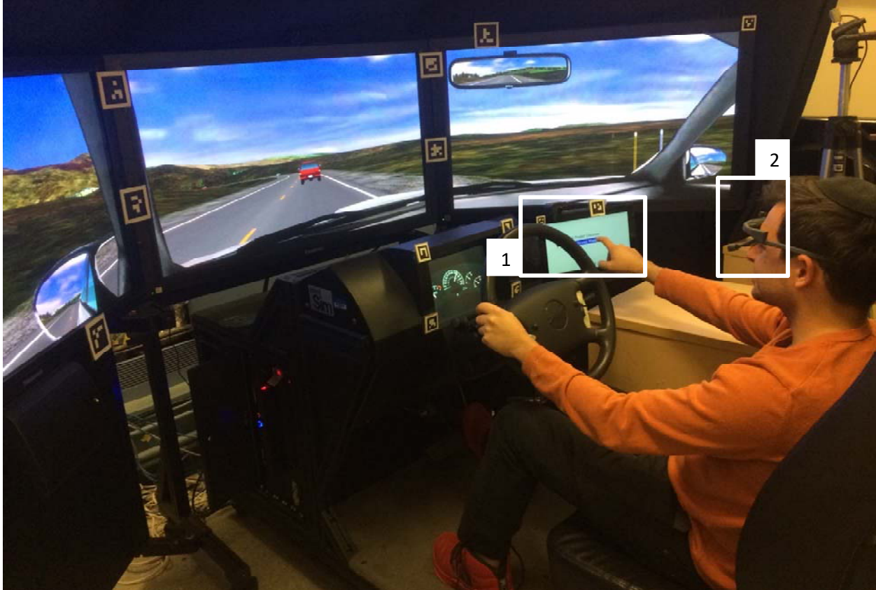
Figure 2: Simulator set up with Surface Pro 2 (1) for the secondary task, and a Dikablis eyetracker (2)
