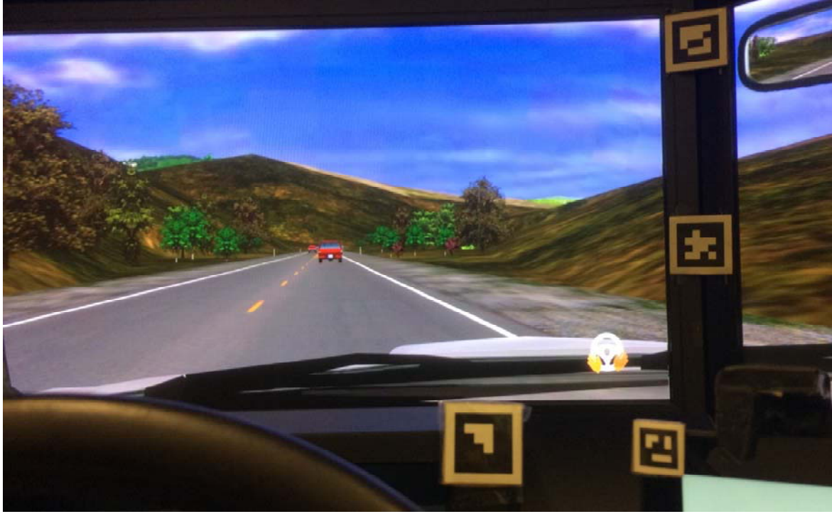
Figure 4: View of TOR display on the center monitor from the perspective of the driver. The TOR is at the bottom right of the screen.
