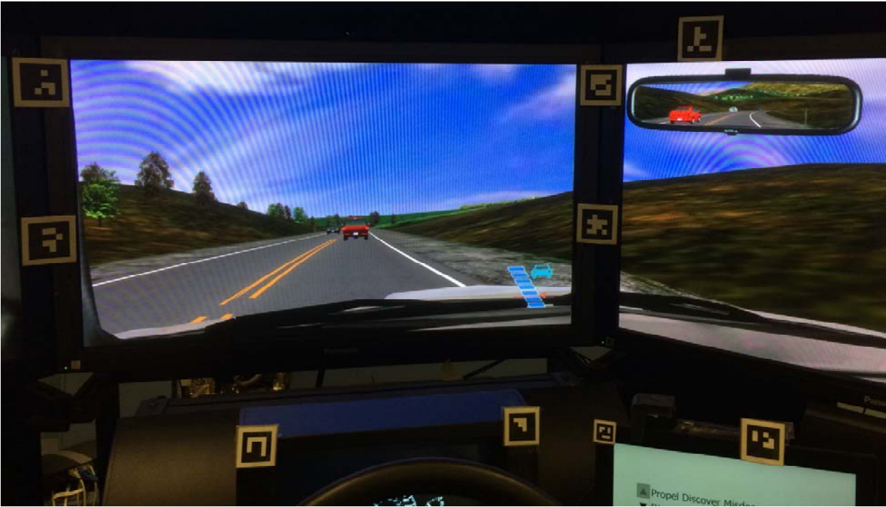
Figure 6: View of the reliability display at Level 7 on the center monitor from the perspective of the driver. The reliability display is at the bottom right of the screen.
