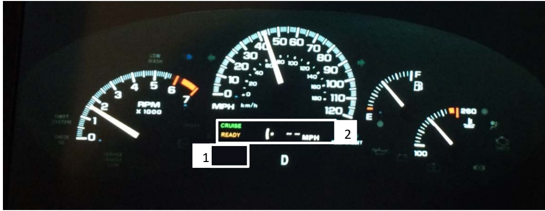
Figure 10: Dashboard display when both the ACC and LK are off. (1) The LK is off, as indicated by the lack of display. (2) the ACC is off, as indicated by no set speed. It also says “cruise ready”, which means that participants can engage the ACC at any point in time.
