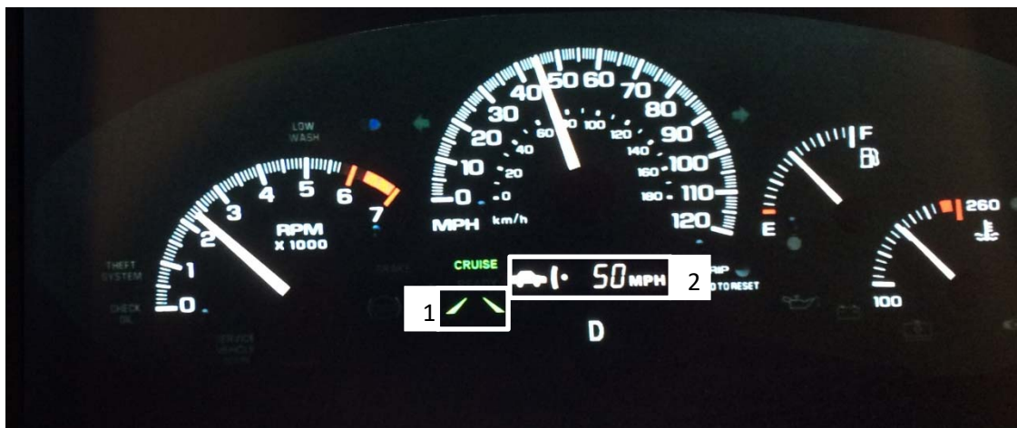
Figure 9: Dashboard display showing the ACC and LK ON. (1) LK is on. (2) The ACC is on, and the set speed is 50 mph. The car indicates that the sensors sense the lead vehicle, and the line and the dot indicate the 3s headway gap that was told to the participants.
