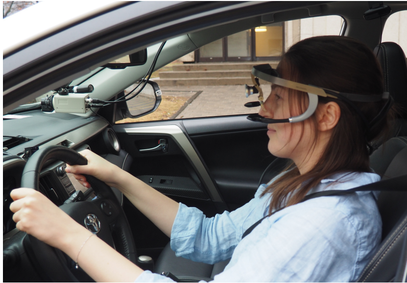
Figure 5: Driver outfitted with Dikablis eye-tracking glasses
