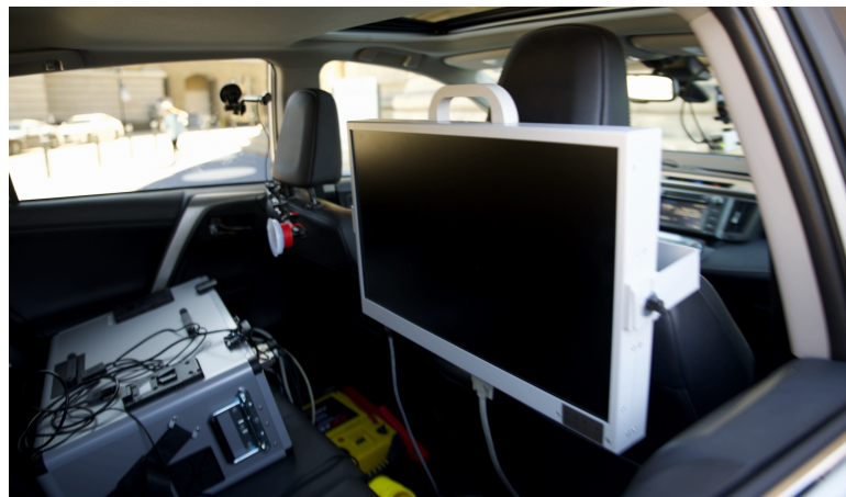
Figure 2: Back seat of the instrumented vehicle
