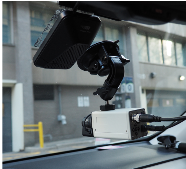
Figure 3: MobilEye and front-facing camera mounted in the vehicle
