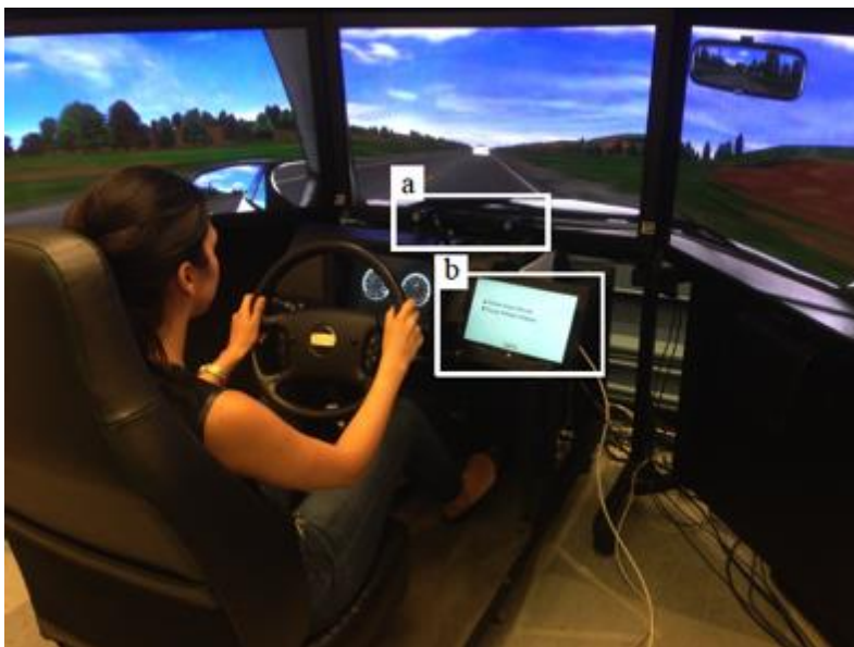
Figure 1: University of Toronto HFASt Laboratory NADS MiniSim™ driving simulator with (a) eye-tracking system and (b) in-vehicle display
