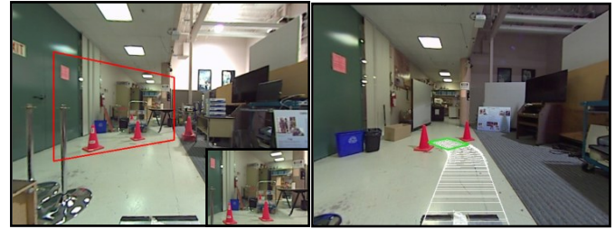
Figure 3 – Projected (left) and Avatar (right) views for the same current rover position and 3-second history.
