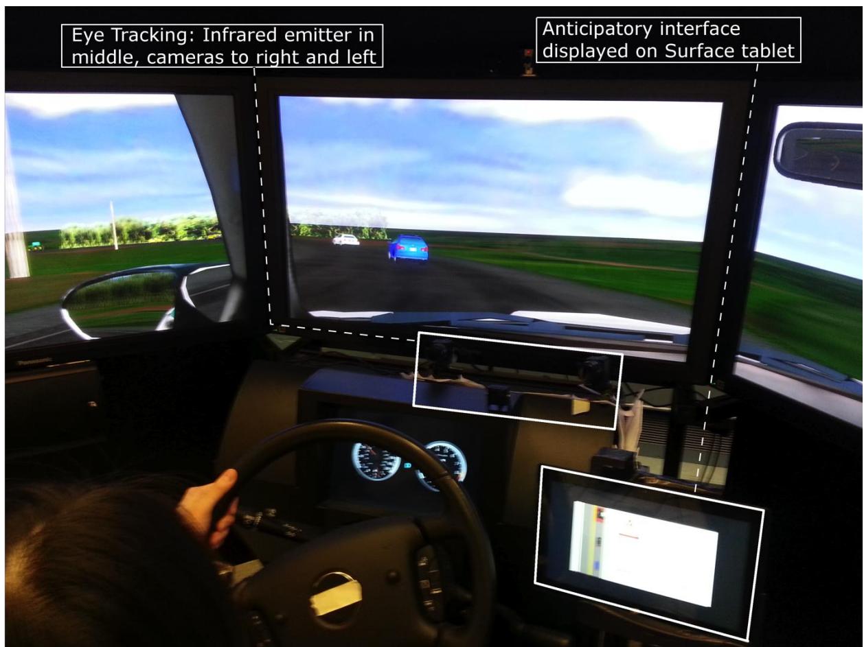
Figure 5: NADS MiniSim driving simulator with FaceLab eye-tracking system and Microsoft Surface
