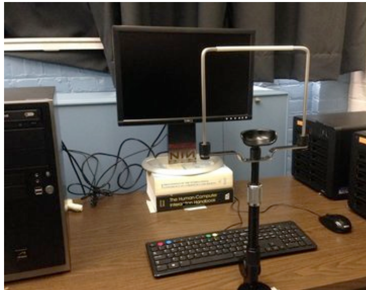
Figure 8: Experimental setup for executive function tasks, including head/chin rest used in the flanker task
