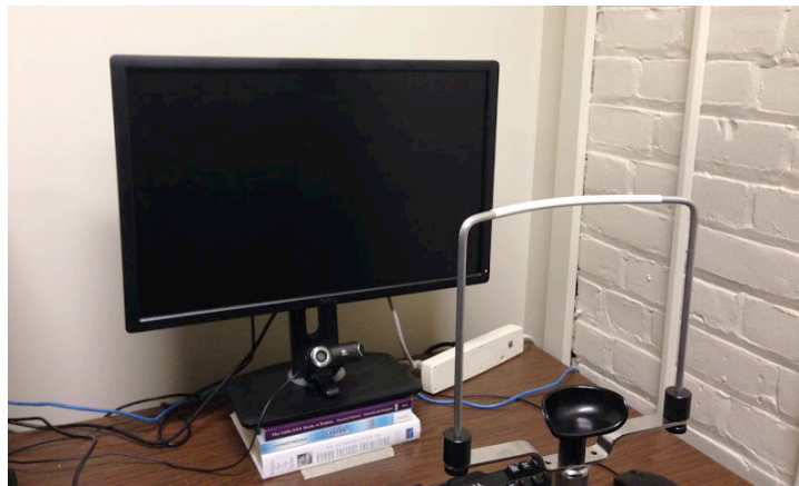
Figure 4: Computer-based attentional task setup, including the head/chin rest
