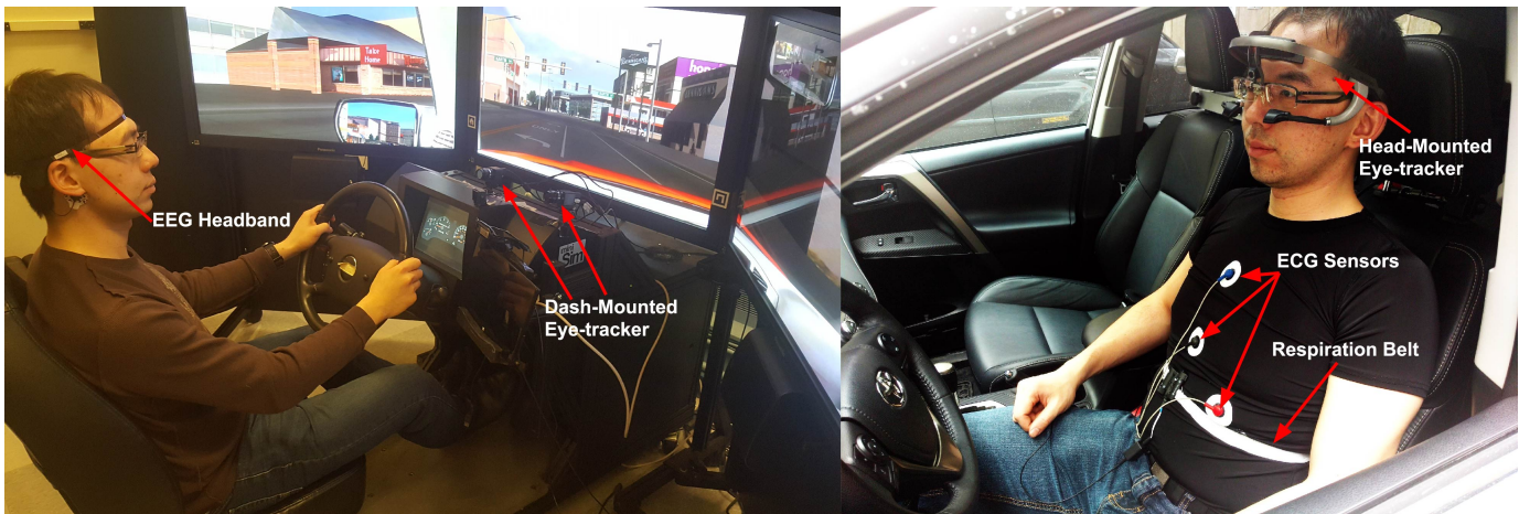
Fig. 4: Example research setup at the University of Toronto for a driving simulator (left) and an instrumented vehicle (right). The simulator shown is a fixed-based simulator, paired with a dashboard mounted eye-tracker. Both the driving simulator and the instrumented vehicle are set up to provide common vehicle measures, including speed, lane position, brake/accelerator pedal position, and headway distance. In the instrumented vehicle, the driver is shown wearing a head-mounted eye-tracker. ECG, GSR, and respiration sensors are also attached to driver's clothing to illustrate potential sensor placement on the participant. For actual data collection, physiological sensors are to be placed directly on skin.
