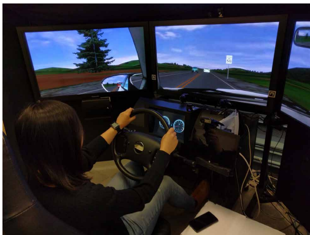
Figure 1. Experiment I apparatus: NADS MiniSim simulator with a Pebble smartwatch on the participant's left wrist and the Nexus 5 smartphone placed to the right of the participant
