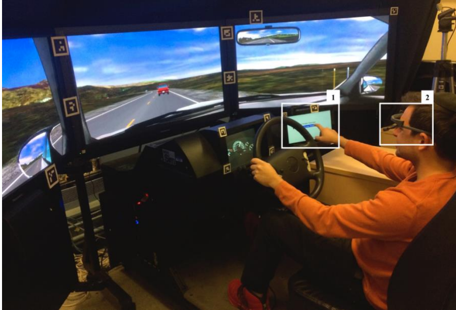
1 2 FIGURE 1: Simulator set up with Surface Pro 2 tablet (1) for the secondary task, and a 3 Dikablis eyetracker (2) 4
